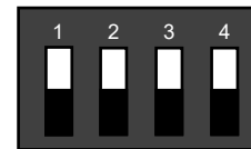
SW1 and SW2 - Setting the IP Address
